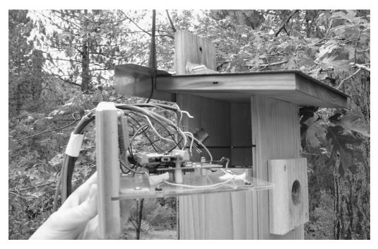
Figure 1.4. Nesting box with interior electronics at James Reserve. This prototype bird box with camera captured and logged still images of bird activity every fifteen minutes, twenty-four hours per day. Photograph by author.
