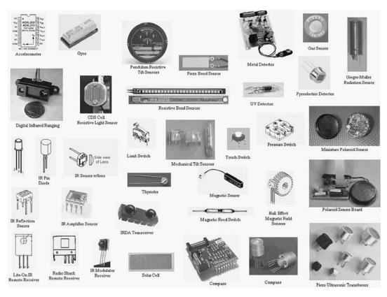
Figure I.3. Types of sensors. Sensors detect and measure stimuli through a wide range of inputs, including chemical, mechanical, and biological sources. The sensor assemblage typically involves using electronics and software to convert stimuli into electrical and digital signals. Screen capture.
