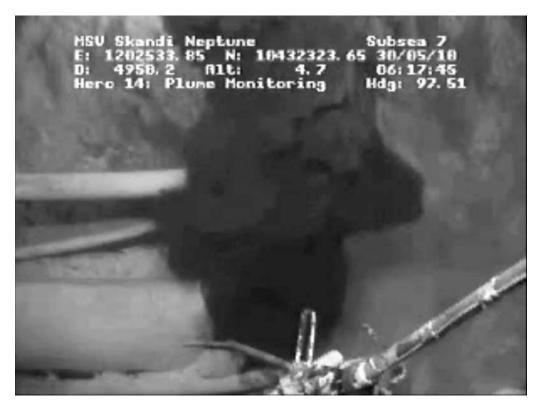
Figure 2.4. Spillcam example footage. BP video from Remotely Operated Vehicle (ROV) monitoring the plume of oil, gas, and mud escaping from the ruptured BP pipe. Screen capture.
