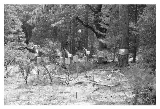
Figure 1.6. An array of sensors at James Reserve measuring moisture and respiration of  $CO_2$  throughout the soil. Photograph by author.
