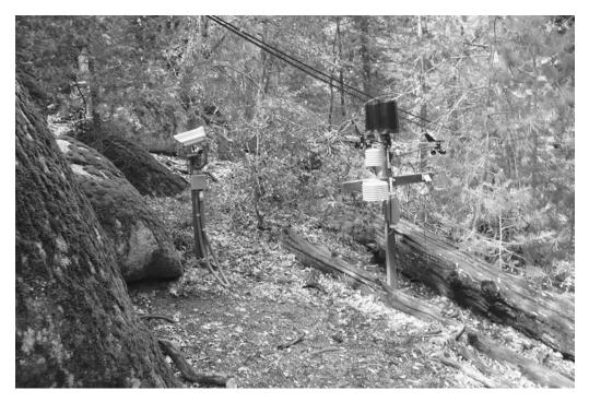
Figure 2.3. Moss Cam with weather station at James Reserve. Image and infrared data are compared to weather observation data to understand the moss lifecycle. Photograph by author.
