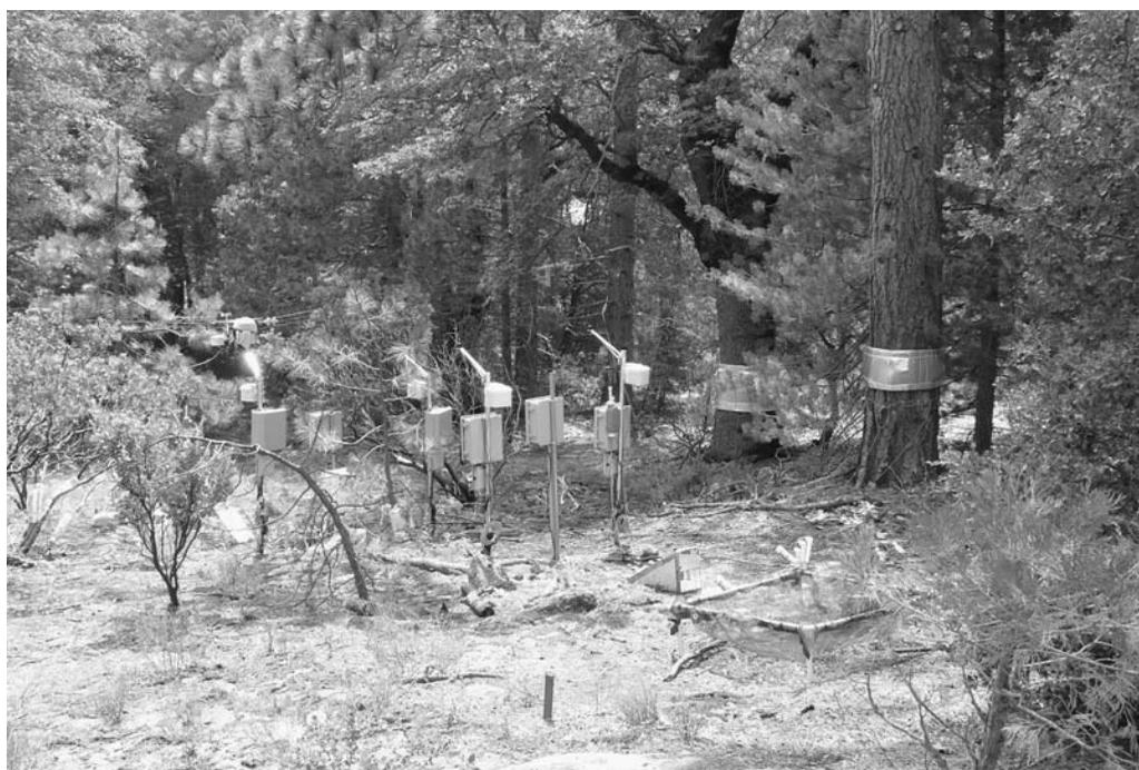
Figure 1.6. An array of sensors at James Reserve measuring moisture and respiration of CO<sub>2</sub> throughout the soil. Photograph by author.
