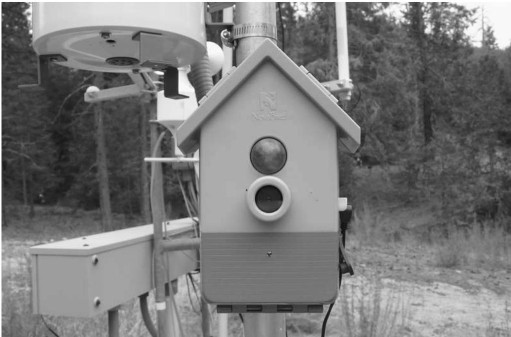
Figure 1.3. Monitoring station with Bird Box Cam at James Reserve. This CENS monitoring station included weather observation as part of its sensing kit and was a test-bed that contributed data to the U.S. National Ecological Observatory Network (NEON). Photograph by author.
