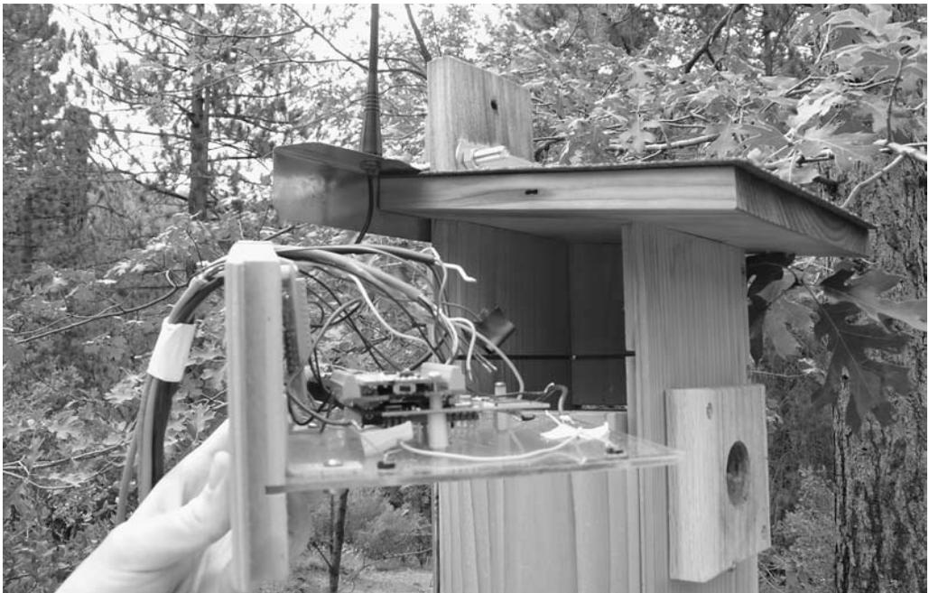
Figure 1.4. Nesting box with interior electronics at James Reserve. This prototype bird box with camera captured and logged still images of bird activity every fifteen minutes, twenty-four hours per day. Photograph by author.
